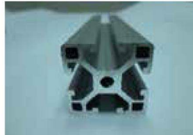
PM-3030 | Aluminum profile 3030 | 30x6000 | 0,801 | AL6063-T5/ MATT NA 10-12uF
