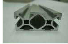
PM-2040 | Aluminum profile 2040 | 20x40x6000 | 0,814 | AL6063-T5/ MATT NA 10-12uF
