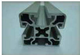
PM-4040 | Aluminum profile 4040 | 40x40x6000 | 1407 | AL6063-T5/ MATT NA 10-12uF
