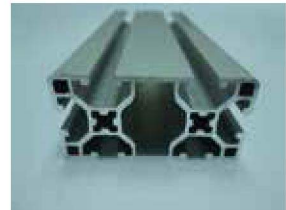
PM-3060 | Aluminum profile 3060 | 3060x6000 | 1371 | AL6063-T5/ MATT NA 10-12uF
